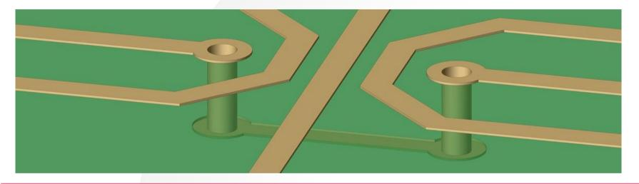
When PCB designers are laying out the PCB tracking, they may come to a point in their design where it is not possible or practical to connect all the tracks to their required origins and destinations. The current method of solving this dilemma is to break through the PCB and continue the track on the underside of the PCB, creating a second copper layer. The two ends are joined with a plated-through hole, called a via.
