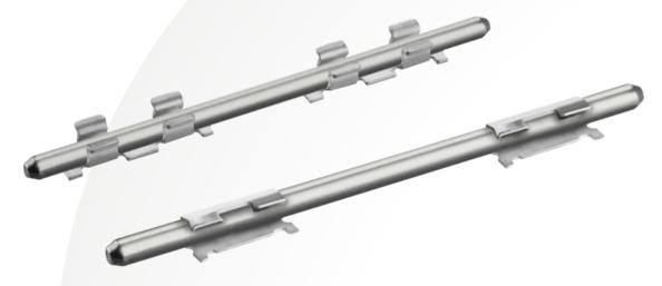
Harwin's novel two-piece combination system of Surface Mount Contacts and a Removable Jumper Link allows manufacturers to connect adjacent PCBs without these problems. The SMT contacts are reflowed to the PCB with all the other components. The Removable Links are then assembled quickly and easily, either in the factory, or even on-site if required.
