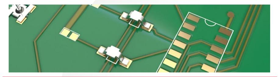
The single piece fixed SMT Jumper Links are a low-cost, easy-to-use solution for track layout problems. Acting as a physical bridge, the designer can simply jump the circuit off the PCB to reach the other side of the problematic track. Vias and double-sided PCBs can be eliminated.
