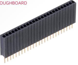
The Archer M52 range include both single and double row options, based on a 1.27mm pitch along the connector. Pitch between rows on the double row is 2.54mm, and male pins are 0.46mm square.
