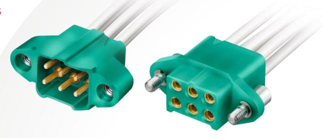
Both Male and Female cable connectors are designed to suit 18AWG to 22AWG equipment wires, with a maximum external diameter of Ø1.8mm for 18-20AWG, and Ø1.4mm max for 22AWG.
