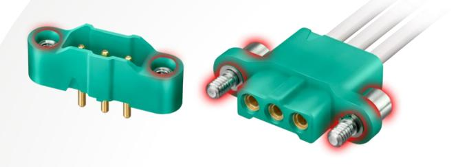
Female crimp connectors are fitted with floating Hex Socket jackscrews, suitable for 2mm Hex (Allen) keys. These will engage with jackscrews assembled in both Male Throughboard and Male Crimp connectors.
