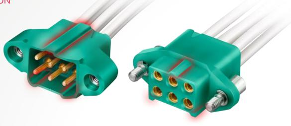
The polarization has been placed on both sides of the connector, to ensure that these connectors cannot be mated inversely. Three polarization keyways have been included in the design, on two corners and in one side.
