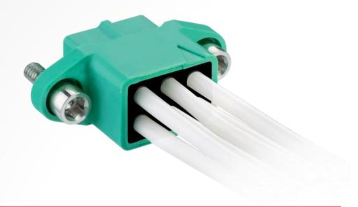
The crimp housings feature a potting wall to keep potting fluids retained during application. The use of potting improves the retention of the crimp contacts in the housing by adding strain relief. The ready-made cable assemblies come with <u>backpotting</u> in place.
