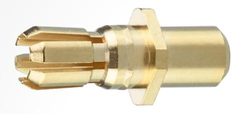
In contrast to the other <u>HRi high-reliability connectors</u> (where the female contact is the heart), here you'll find a 6-fingered Beryllium Copper male contact providing a positive normal spring force against the female mating contact. The durable hard-acid gold finish ensures repeated mating cycles and long-term environmental exposure do not affect the connection surfaces.
