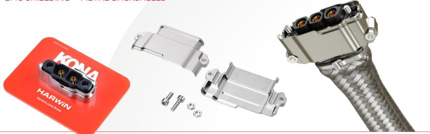
The strong and lightweight machined <u>aluminium backshells</u> provide additional strain relief. They are designed to accommodate flexible, abrasion resistant, metal braiding and are supplied with tie-bands to attach such braiding to the shell. The backshells, together with the braiding, provide shielding for enhanced electrical continuity and effective EMI/RFI protection.
