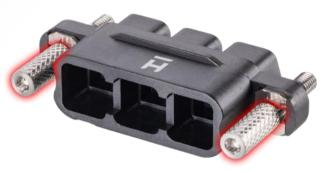
All Kona connectors are fitted with screw-lock fixings, to achieve the maximum vibration and shock specifications. They are also mate-before-lock, so connectors are easier and faster to mate before the screws are engaged and screwed together.
