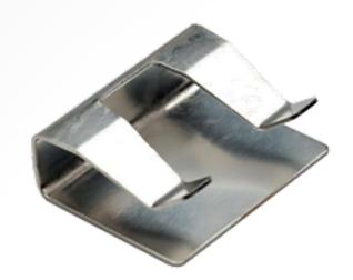
Available in 5 sizes, with the smallest having a footprint of 5.5mm x 4.5mm and a height of only 1.5mm, these Surface Mount Cable Clips are suitable for managing multiple cables from 0.9mm up to 3mm diameter. The complete range can be found on the website, and samples can be requested from the individual Product pages.
