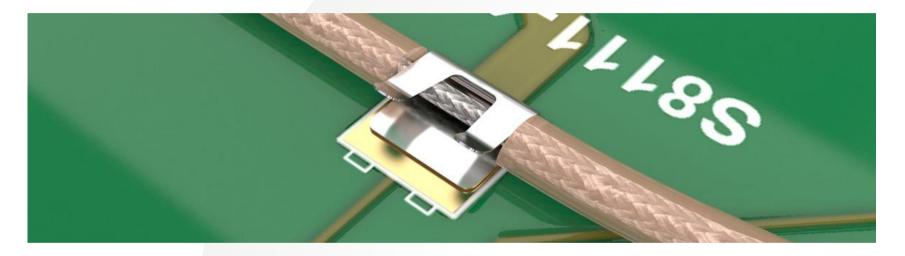
The unique metal construction used in a Cable Clip allows the conductive properties of the part to be utilized. By acting as a direct electrical connection to a PCB ground plane, this provides a novel and cost-effective means of connecting coax screening braid directly to ground with no additional parts or costs.
