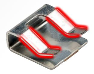
The unique metal dual beam design provides a secure, easy and flexible retention to the cables. The retaining features provide a large lead-in for the cables, making it easy to install the cables into the clips.
