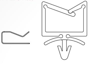
As electronic component density increases, PCB space becomes increasingly premium. These spring metal clips provide maximum cable capacity in the lowest possible profile, especially when compared to the plastic alternatives. Automated placement to the PCB permits easy orientation of the clips, making them ideal for use where close management of a cable run is required.
