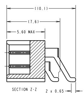
SPECIFICATIONS: MATERIAL: MOULDING = GLASS-FILLED PPS, UL94V-O, BLACK CONTACT = COPPER ALLOY IOILOK RETAINER = STAINLESS STEEL FINISH: 22 = 0.75µ GOLD ON CONTACT AREA, 3µm 90/10 TIN/LEAD ON TAILS 42 = 0.75µ GOLD ON CONTACT AREA, 3µm 100% TIN OVER NICKEL ON TAILS CURRENT RATING AT 25°C = 3.0A MAX CURRENT RATING AT 85°C = 2.2A MAX WORKING VOLTAGE = 120V AC/DC
