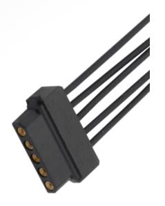
Datamate PIHR is compatible with all female Datamate L-Tek connectors with the same contact arrangement. The 4-fingered Beryllium Copper female contact gives superb performance, for both electrical and mechanical specifications. This inner "contact clip" is stamped and plated with a durable gold finish at our UK headquarters. The spring performance of the contact gives the environmental resistance to shock and vibration, with a temperature range up to 125°C.
