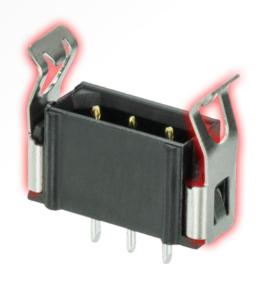
The Datamate L-Tek connectors use simple locking latches made from high strength Beryllium Copper. Mating is fast and simple – just push the two connectors together, and the latches snap into place. The connectors are then locked together and require manual deflection of the latches to separate.
