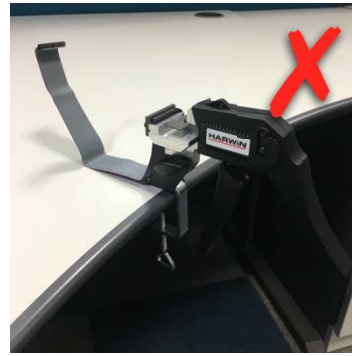
Figure G - Incorrect Position
