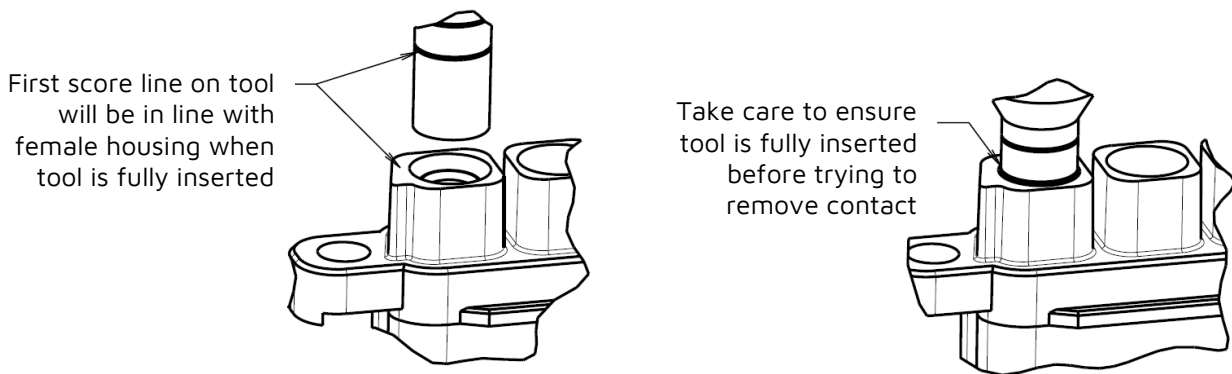
Figure J: Female Contact Removal
