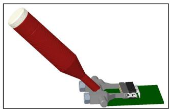
The connectors will de-latch, and the female housing will remain between adjustable jaws of tool as shown.
