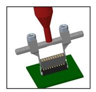
To remove female connector from the adjustable jaws they will need to be separated by hand. Only one jaw will need to be moved to release the female connector.
