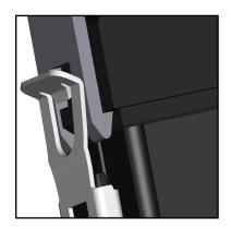
With the de-latching tool engaged with the female housing, the connectors are now ready to be separated. Ensure a steady pulling force is applied to the tool; perpendicular to the PCB for vertical connectors and parallel to the PCB for horizontal connectors.
