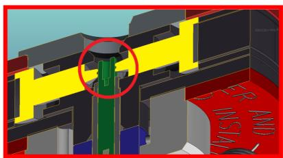
If the plunger is not fully home, the indentors could crimp on the plunger, damaging both the Z125-900 hand tool and the Z125-901 positioner {Figure H}.
