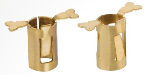
Previous designs of SMT contacts have only included 2 points of contact to the mating pin, making them potentially vulnerable to vibration. The Sycamore Contact patented design incorporates 3 points of contact for improved continuous signal integrity.
