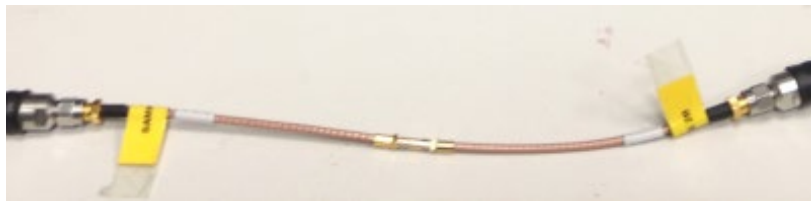
Typical test cable assembly with mated M80-307 and M80-317 coax contacts
