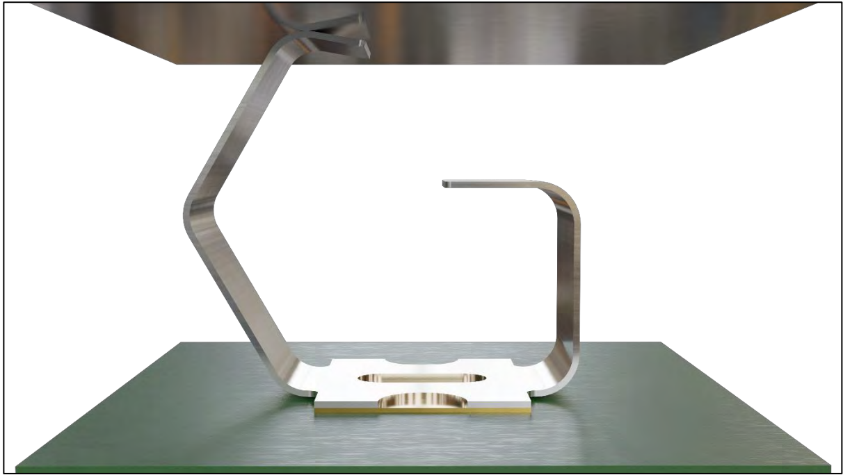
Figure 1: Vertical Compression of a Multi-Directional Spring Contact
