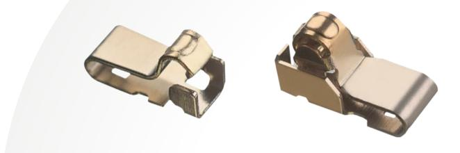
A further development of the extended C style, these contacts were originally designed for wireless antenna connections on many mobile devices, such as smartphones, or LED lamp connection and RFID tags. The Positive Stop shoulder prevents the contact from being over-compressed, which can lead to permanent set and a reduction in spring force.
