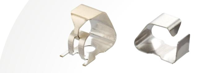
Box style contacts are different to the C style by the addition of a feature that reduces the risk of damage caused by accidental snagging. On some Box designs, it also prevents unwanted lateral movement of the contact during mating. This style can also be labelled as Anti-Hooking.
