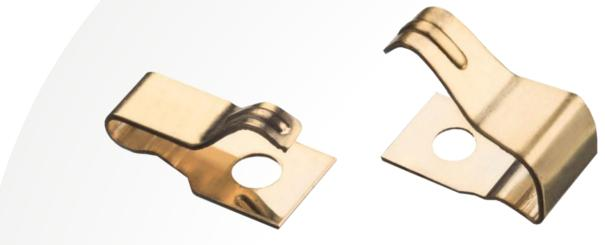
A development of the C style contact, this design uses a more obvious cantilever style. The SMT pick and place area is exaggerated to compensate for the miniature size of the contact. This range is provided in 0.5mm incremental step heights, from 2mm up to 5mm. The footprint is the same across the complete set of contacts.
