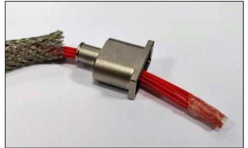
3. Remove the tape on the cable bundle end.
