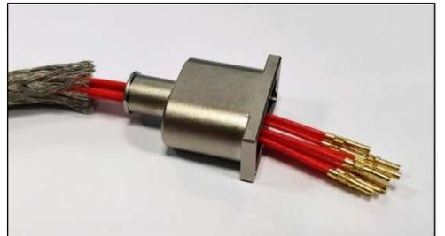
5. Insert the individual contacts into the connector housing.
