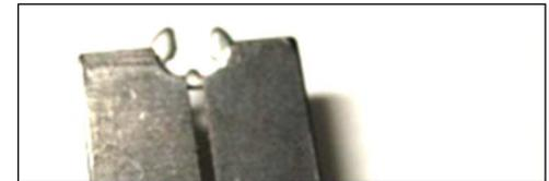
8. Assemble the E-Clip onto one of the jackscrews.
