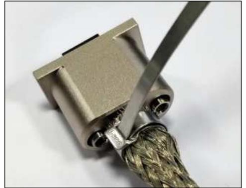
11. Use the BAND-IT tool on the tie to secure it on the braid and backshell.
