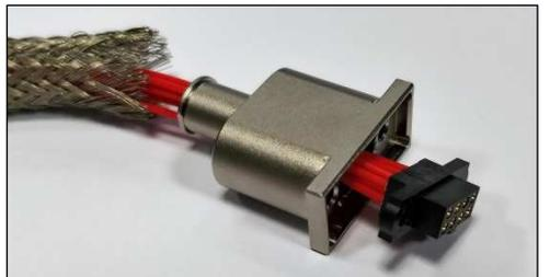
6. Push the completed connector fully into the backshell. Assemble the jackscrews through the rear of the backshell.
