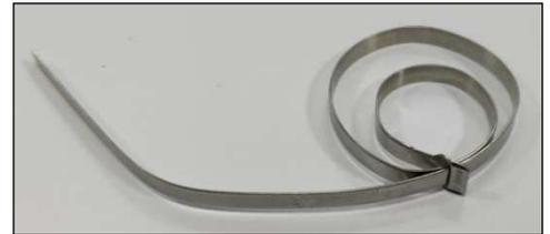
Pull it hand-tight, making sure that the buckle is sitting on the long side of the elliptical rear exit.
